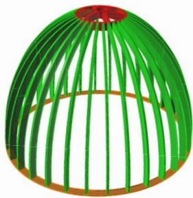
Exterior Elliptical Dome
